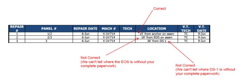
2. When providing panel dimensions in your field book and on the drawing, remember to provide all of the required dimensions and notes. (If there is no room on a single page, start a new one and reference back to the original notes.)
